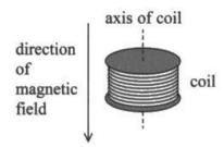
The coil was rotated through 90° so the axis was perpendicular to the direction of the field, as shown.
