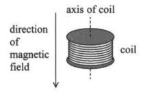
The coil was rotated through 90° so the axis was perpendicular to the direction of the field, as shown.
