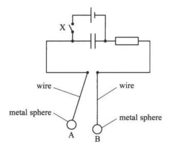
When the wires hang vertically the spheres are in contact and the discharging circuit is complete.
