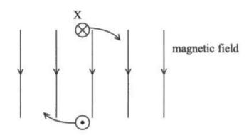
The coil is rotated clockwise in the magnetic field, causing a current in the coil. The student states that the current at X is into the page.
